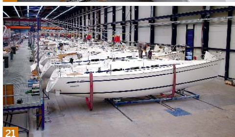
21 The end of the line. Upholstered cushions are added and several quality-control checks are completed. Notice the blue rack on which the last boat has been riding up the line. Each rack collapses flat and is attached to a cable in the floor (notice the blue square on the floor) that pulls the entire line in unison. When the boat comes off the end of the line, the rack is returned to the beginning of the line via a cable under the raised work area behind the line.
