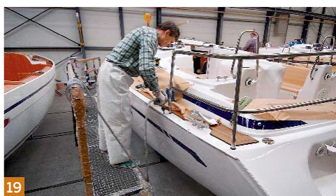
19 The joint is then screwed down with stainless-steel screws every 4 inches forming the mechanical bond; the interior of the joint is glassed over and the toerail is installed.
